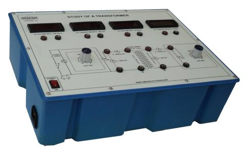
**OMEGA TYPE ETB-110** Experimental Training Board has been designed specifically for the study of a Transformer. Various measurements can be easily done on a transformer. The board is absolutely self contained and requires no other apparatus.
