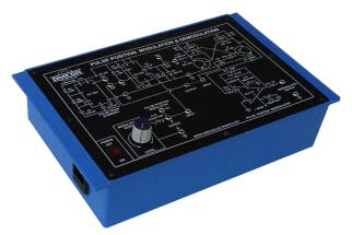
**OMEGA TYPE ETB-114** Experimental Training Board has been designed specifically for the study of Pulse Position Modulation and Demodulation. Using this training board one can know the specialized techniques of Pulse Position Modulation and Demodulation.
