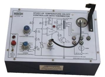
**OMEGA TYPE ETB-148** Experimental Training Board has been designed specifically to study the principle of Temperature Control with the use of a Thermistor. This is one of the important industrial applications of the thermistor. The board is absolutely self contained and requires no other apparatus.
