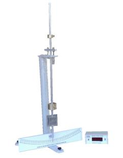
OMEGATYPE ES-391 Experimental Set Up has been designed specifically to study the damping using a compound pendulum. The set up is absolutely self contained and requires no other apparatus.
