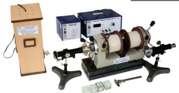
**OMEGA TYPE ES-367** Experimental Set-Up has been designed specifically to study the Faraday Effect and hence to determine the Verdets Constant for a given substance.
