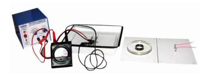
OMEGA TYPE ES-368 Experimental Set-Up has been designed specifically to sketch the two Dimensional Potential Mapping for various configuration. The set-up consist of Parallel Plates, Co-axical Cylinder, infinite rods, container tray etc.
