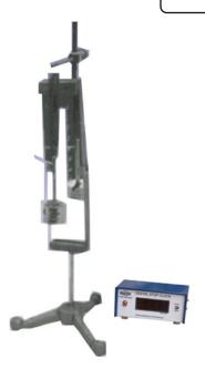
**OMEGA TYPE ES - 373** Experimental Set-Up has been designed specifically to find the spring constant of a helical spring from the load extension graph by hook's law.
