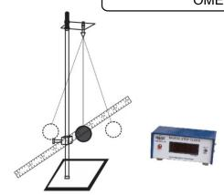
OMEGA TYPE ES - 374 Experimental Set-Up has been designed specifically to study of damped simple harmonic oscillation & determination of damping coefficient of damping, relaxation time & quality factor using simple pendulum
