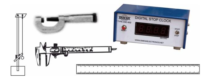
OMEGA TYPE ES - 376 Experimental Set-Up has been designed specifically to Study the Torsion. of Wire, its Dependance on Radius, Length Torque and Material of wire & to determine the modulus of rigidity of the material of wire with the help of torsional pendulum.
