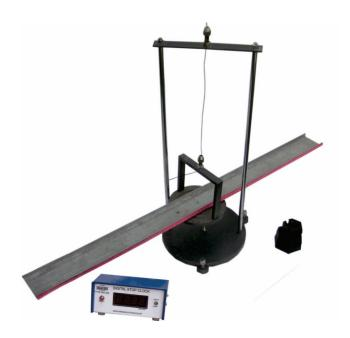
**OMEGA TYPE ES - 379** Experimental Set-Up has been designed specifically to study the law of parallel axes for moment of inertia
