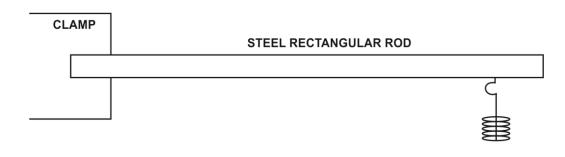
**OMEGA TYPE ES-380** Experimental Set-Up has been designed specifically to study the cantilever bending : different loading positions & other parameters.
