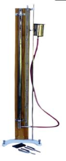
**OMEGA TYPE ES - 381** Experimental Set-Up has been designed specifically to determine the velocity of sound in air with the help of a resonance column using three tuning forks and to plot a graph between the frequency and the resonating length.
