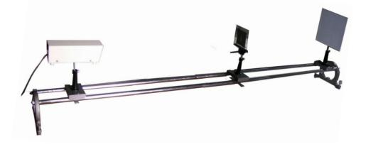
**OMEGA TYPE ES-388** Experiment set-up has designed specifically for Demonstrations of Interference and Diffraction Phenomena Using Laser. The Set up is absolutely self-contained and requires no other apparatus. Practical experience on this set up carries great educative value for Science and Engineering Students.
