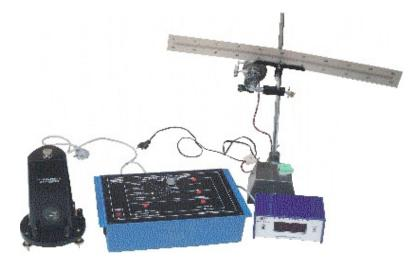
**OMEGA TYPE ES-389** Experimental Set-Up has been designed specifically to determine the high resistance by leakage method by means of a Ballistic Galvanometer.
