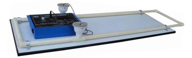
**OMEGA TYPE ES-395** Experimental Set Up has been designed specifically for To study and determine the velocity of sound in air using the quincke's tube method at room temperature.
