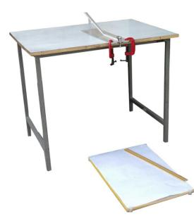
OMEGA TYPE ES 397:- Experimental Set Up has been designed specifically for to study the conservation of momentum in two dimensional collision.
