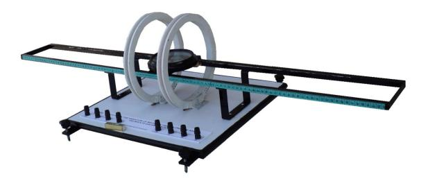
**OMEGA TYPE ES-399** Experimental Set-up has been designed specifically to study the variation of magnetic field along the axis of helmholtz galvanometer
