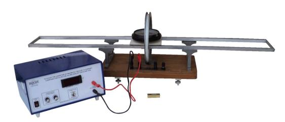
**OMEGA TYPE ES-392** Experimental Set-up has been designed specifically to study the variation of magnetic field by a current carrying circular coils along axis of circular coil Draw necessary graph for it and find the radius of the coil
