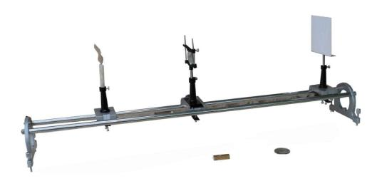
OMEGA TYPE ES-408 Experimental Set Up has been designed specifically to study the nature and size of the image formed by a convex lens / concave mirror on a screen by using a candle and a screen (for different distances of candle from the lens).
