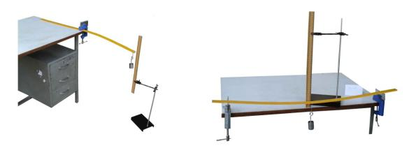
**OMEGA TYPE ES-410** Experimental Set Up has been designed specifically for studying the effect of load on depression of a suitably clamped loaded meter scale.
