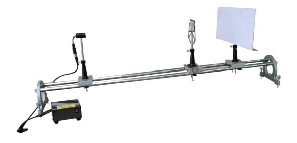
**OMEGA TYPE ES-413** experimental set-up has been designed specifically to determine the number of lines per centimetre on a diffraction grating.
