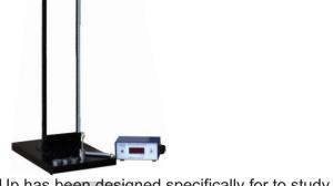
OMEGA TYPE ES-396 Experimental Set Up has been designed specifically for to study of oscillations for a mass and determine the force constant in different case's.
