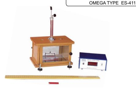
OMEGA TYPE ES-411 Experimental Set-up has been designed specifically to verify the force ratio of end on position to broad on position of a bar magnet.
