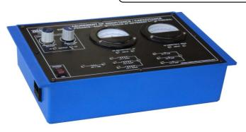
**OMEGA TYPE ES-412** Experimental Set-up has been designed specifically to measure inductance / capacitance using impedance at different frequencies..
