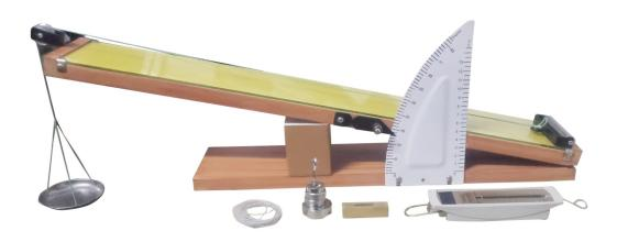
OMEGA TYPE ES-429 Experimental Set Up has been designed specifically specifically to find the downward force, along an inclined plane, acting on a roller due to gravity and study its relationship with the angle of inclination by plotting graph between force and  $\sin \theta$ .
