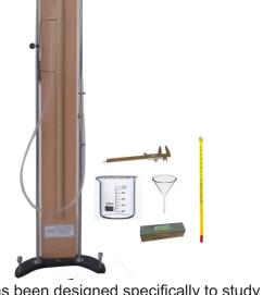
**OMEGA TYPE ES-430** Experimental Set Up has been designed specifically to study the variation in volume (V) with pressure (P) for a sample of air at constant temperature by Boyle's law by plotting graphs between P and V and between P and 1/V.
