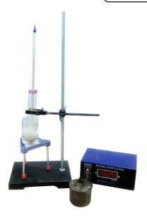
OMEGA TYPE ES-432 Experimental Set Up has been designed specifically to observe the change of state and plot a cooling curve for molten wax.
