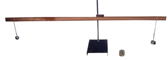
**OMEGA TYPE ES - 435** Experimental Set Up has been designed specifically to determine the mass of a given body using a metre scale by the principle of moments.
