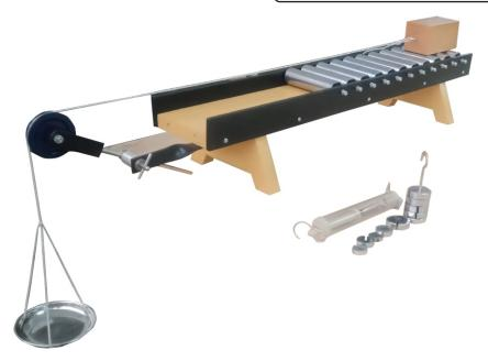
**OMEGA TYPE ES - 436** Experimental Set Up has been designed specifically to measure the force of limiting rolling friction for a roller (wooden block) on a horizontal plane.
