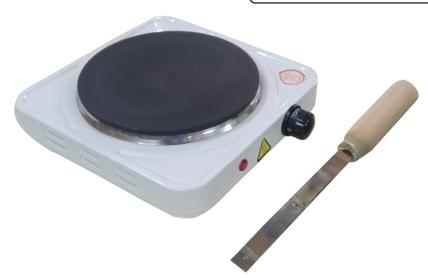
OMEGA TYPE ES - 439 Experimental Set Up has been designed specifically to observe and explain the effect of heating on a bi-metallic strip.
