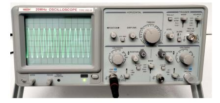
**OMEGA TYPE CRO-20** This Oscilloscope is corresponding to horizontal style with small size. The bandwidth of Y axis is DC~20MHz and the deflection factor is 5mV~5V/DIV. It can be up to 50V/DIV supplying with the 10.1 probe. Sweep deflection factor is 0.1us/div-0.1s/div. It has the Following features wide measurement, high sensitivity trigger lock and etc. Sweep switch adopt code switch and accuracy orientation. It is convenient to operate.
