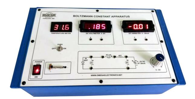
**OMEGA TYPE ETB-285** Experimental Training Board has been designed specifically for to Determine the Boltzmann Constant and V-I Characteristics of PN Junction Diode
