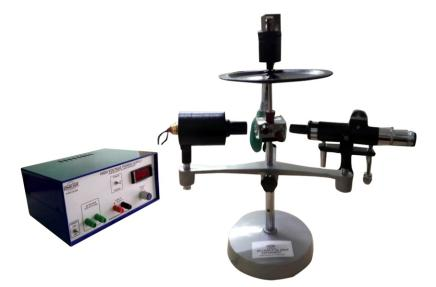
**OMEGA TYPE ES-450** Experimental Set-Up has been designed specifically to determine the charge of an electron by Millikan's oil drop experiment.
