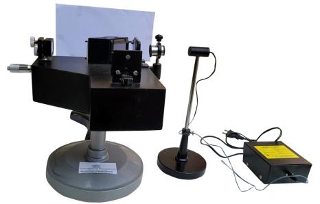
**OMEGA TYPE ES-453.2** Experimental Set-Up has been designed specifically to determine the wavelength of laser source using Michelson's interferometer.
