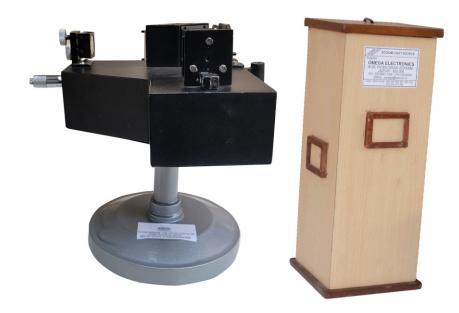
**OMEGATYPE ES-453.3** Experimental Set-Up has been designed specifically to determine the wavelength of sodium light source using Michelson's interferometer.
