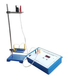
**OMEGA TYPE ES-415** - Experiment set up has been design specifically for determine 'g' and velocity for a freely falling body using digital timing technique. The board is absolutely self contained and requires no other apparatus.
