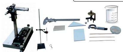
OMEGA TYPE ES-418 Experimental Set Up has been designed specifically to Measurements of Length (Or Diameter) Using Vernier Caliper, Screw Gauge, Spherometer and Travelling Microscope
