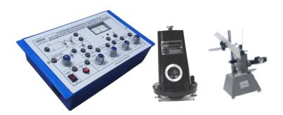
**OMEGA TYPE ES-419** Experimental Set Up has been designed specifically to determine resistance of a galvanometer by half deflection method and study of variation of logarithmic decrement with series resistance using ballistic galvanometer.
