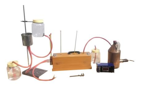
OMEGA TYPE ES-421 Experimental Set Up has been designed specifically to determine the coefficient of thermal conductivity of a metal, by using Searle's apparatus.
