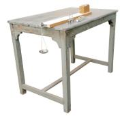
**OMEGA TYPE ES-428** Experimental Set Up has been designed specifically to study the relation between force of limiting friction and normal reaction and to find the coefficient of friction between surface of a moving block and that of a horizontal surface.
