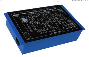
**OMEGA TYPE ETB-115** Experimental Training Board has been designed specifically for the Comparative study of Common Emitter (CE), Common Base (CB) and Common Collector (CC) Transistor Amplifiers. These practical transistor amplifier configurations are evaluated in respect of their main parameters and results are compared with theoretical calculations.
