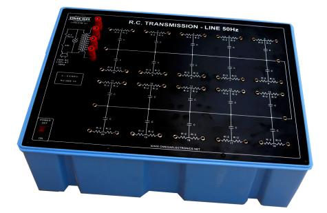
**OMEGA TYPE ETB-127** Experimental Training Board has been designed specifically for the study of R.C. Transmission Line at 50Hz. The variation in magnitude and phase of the voltage after every section can be studied for different input voltages at 50 Hz. One will observe the phase shift of almost 2p in 20 sections.
