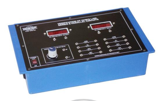
**OMEGA TYPE ETB-128** Experimental Training Board has been designed specifically for the verification of Ohm's Law & to study the series and parallel combination of Resistance network. This training board is quite useful for imparting the basic knowledge of voltage and current distribution and the effect of series parallel circuit. The board is absolutely self contained and requires no other apparatus.
