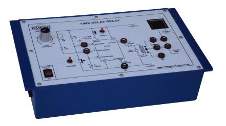
**OMEGA TYPE ETB-124** Experimental Training Board has been designed specifically for the study of Time Delay Relay circuit. This training board can also be used as a time delay relay to control external loads. The board is absolutely self contained and requires no other apparatus.
