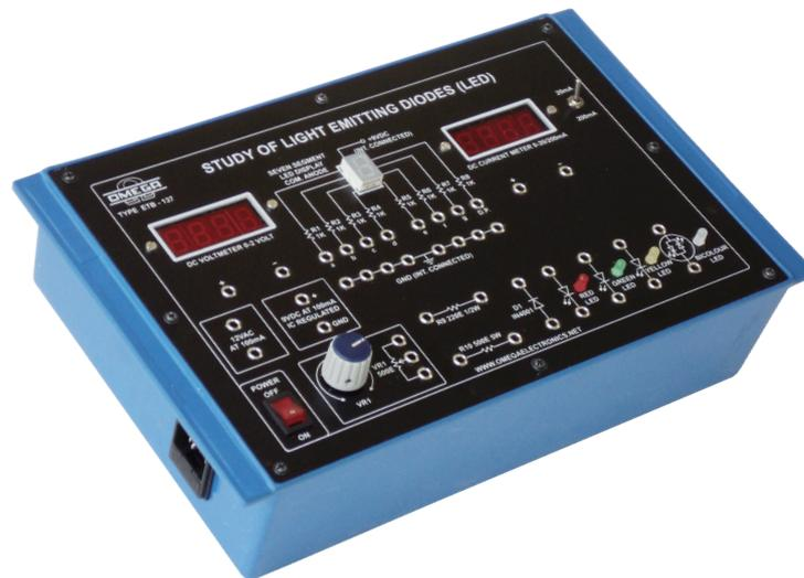
**OMEGA TYPE ETB-137** Experimental Training Board has been designed specifically for the study of Light Emitting Diodes (LED's). The application of an LED as a seven segment display is experimentally explained. The board is absolutely self contained and requires no other apparatus.
