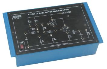
**OMEGA TYPE ETB-138** Experimental Training Board has been designed specifically for the study of Darlington Pair Amplifier.
