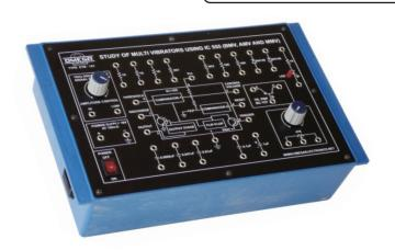
**OMEGA TYPE ETB-141** Experimental Training Board has been designed specifically for the study of Bistable, Astable and Monostable Multivibrators using IC 555.
