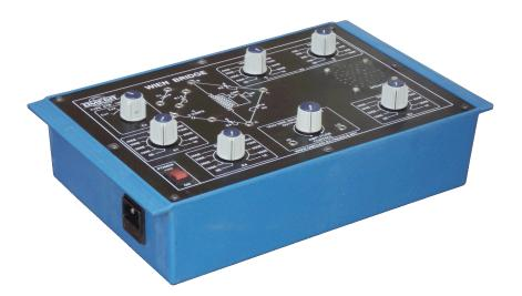
**OMEGA TYPE ETB-136** Experimental Training Board has been designed specifically for the study of Wien Bridge and by which one can evaluate the unknown value of capacitance.
