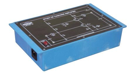
**OMEGA TYPE ETB-147** Experimental Training Board has been designed specifically for the study of Cascode Amplifier. Various parameters of a Cascode Amplifier can be measured on this training board.
