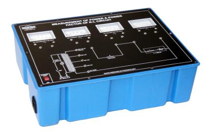
**OMEGA TYPE ETB-149** Experimental Training Board has been designed specifically for the Measurement of Power and Power Factor of R-L Circuit with a single phase of AC voltage source using voltmeters, current meter and a wattmeter.
